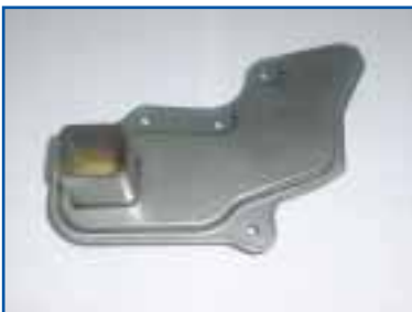
R4AEL (RE4R01A) (Filter has 2" pick-up tube)
