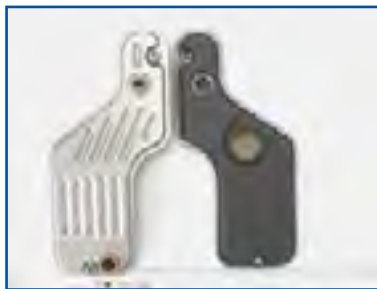
5R110W (External Cartridge w/ O-ring)
